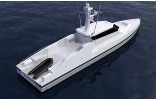
Interceptor model, a high speed vessel of 32 meters for maritime security, designed by CMN with CATIA
