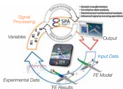
Figure 1. Workflow of SPA highlighting its interaction with both experimental and FE data.
